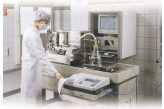
SARTOFLOW® benchtop cross flow filtration unit
